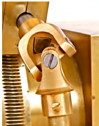
After: Restored/new brass swivels, brass control rods and knobs.
