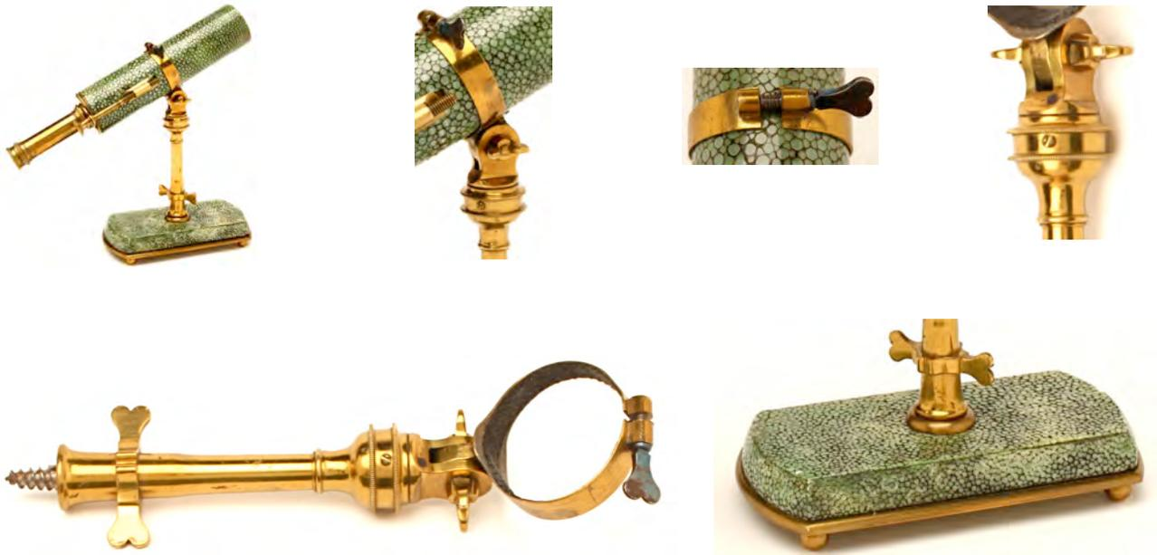
Novel use of a field wood-screw to hold the tripod column to the shagreen-covered brass base
