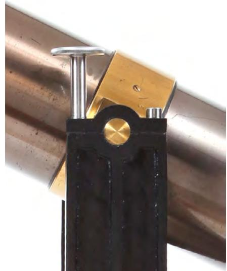
FRE1: SECRETAN Altitude and azimuth adjustment by manually tilting and turning the main tube, respectively.
