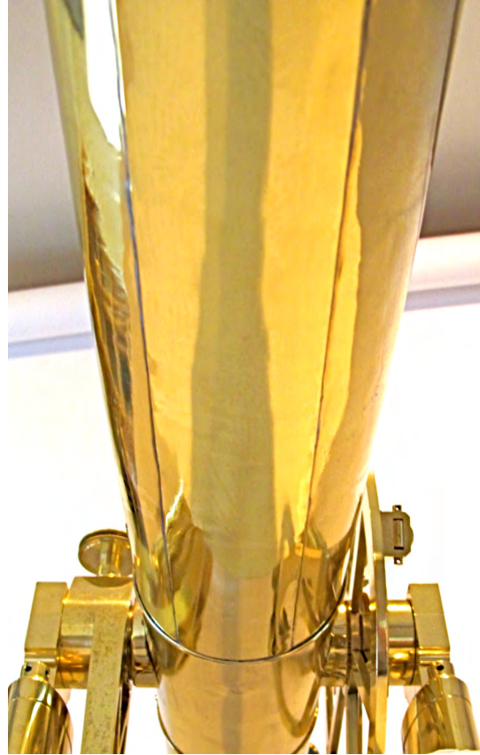
After - showing lower end of the upper tube with its full-length brass patch used to seal a 5-inch long (couple of mm wide) split in the tube seam. Also note the removal of the useless non-original mounting bolts and knurled fasteners
