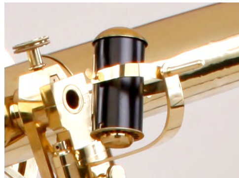
Oil lamp is gimbaled-mounted at the pivot on the transit mount and mid-point on the OTA
