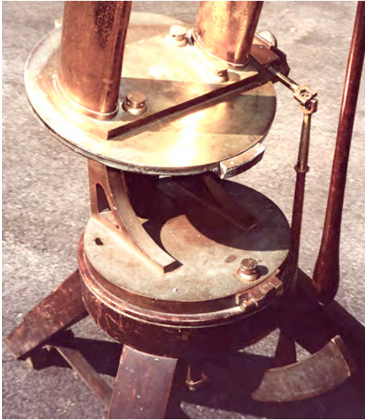
Mahogany tripod base supporting transit trunnions mounted on a large tiltable universal equatorial plate
