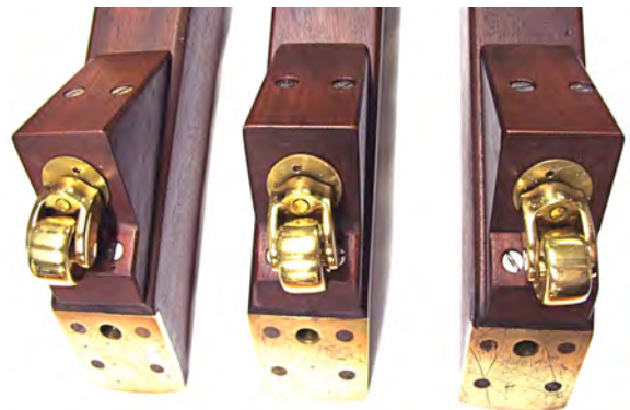
New solid brass casters mounted on heavy mahogany mount blocks required for the 350 lb. load (> 100lb./caster)
