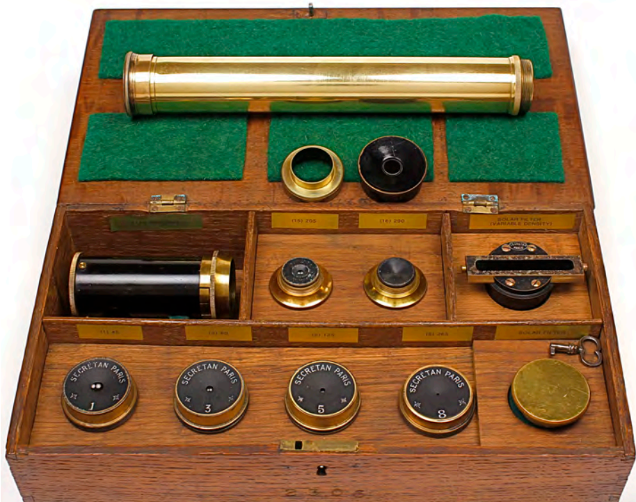
Optical components: lens set, star diagonal, variable and fixed density solar filters, and terrestrial eyepiece. All mounted, except terrestrial eyepiece in a fitted period oak case with key.
