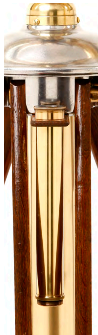
"Hanging" terrestrial eyepiece superimposed in front of the larger diameter central brass elevator tube for raising and lowering telescope.
