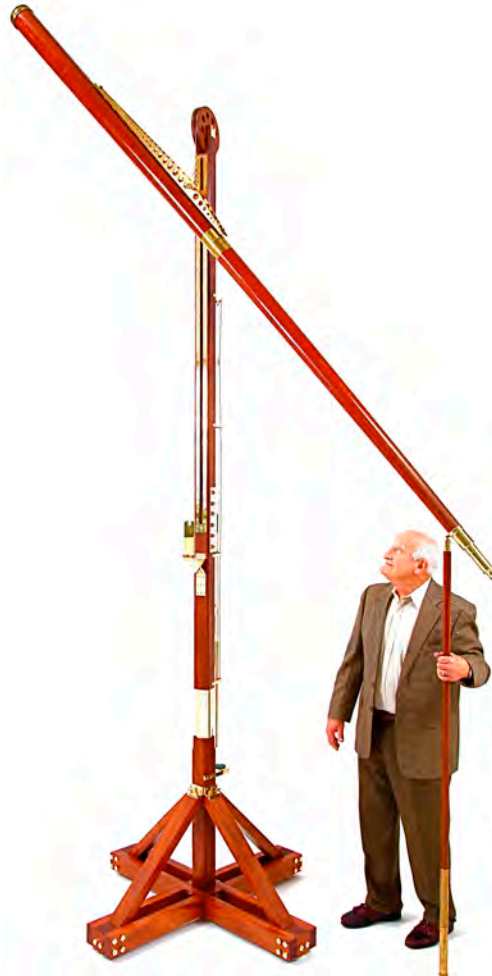
Ed Wolf standing beneath his 12-ft. long Dollond. Custom mahogany pole-and-rope trapeze mount with 30-lb. brass counterbalance (out of view).
