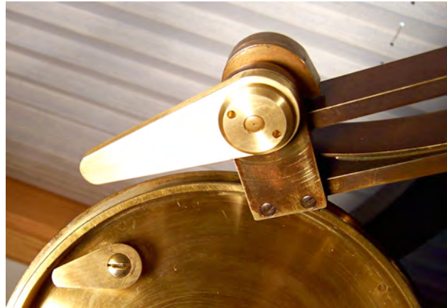
Replaced missing lever and keeper nut (twist tab on main tube lid was used for designing shape of lever)
