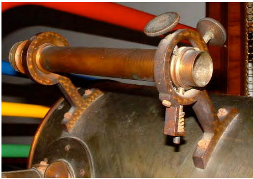
Replaced missing lever and keeper nut (twist tab on main tube lid was used for designing shape of lever)
