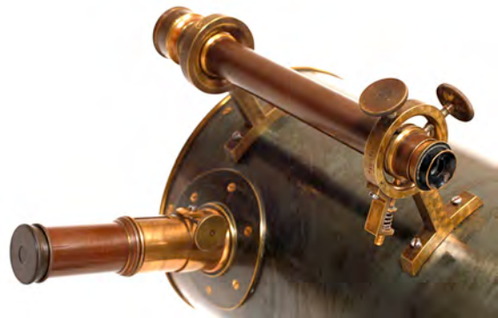
Replaced missing eyepiece in finder scope
