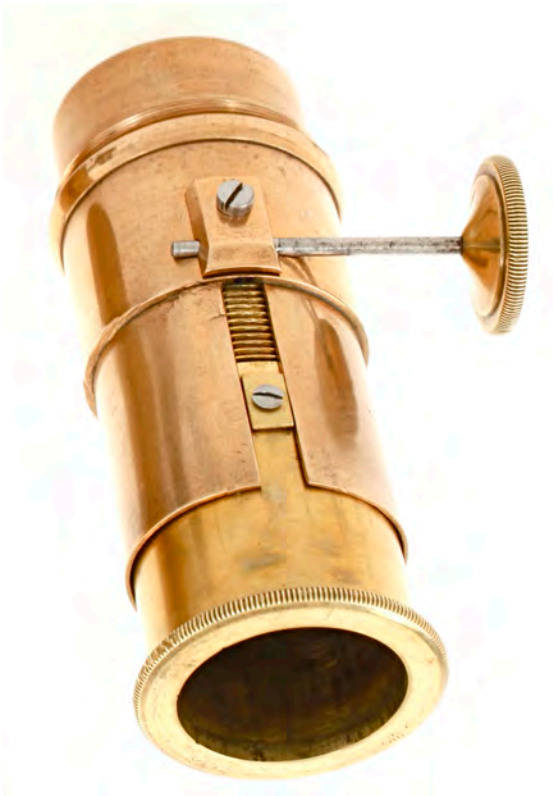
Left: Rack-and-pinion focus mechanism for the ocular lenses.
