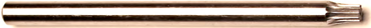
Used very small Rush Gear, Inc., pinion wire to replace old stripped gear: 10 teeth, shaft O.D. = 2.1mm, and gear O.D. = 3.3mm.
